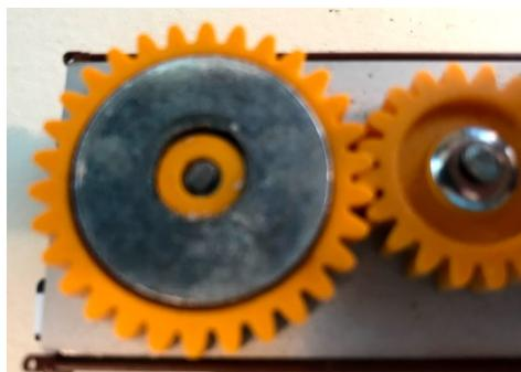
Glue a metal disc onto the gear-wheel to carry the camera - check that it is magnetic
