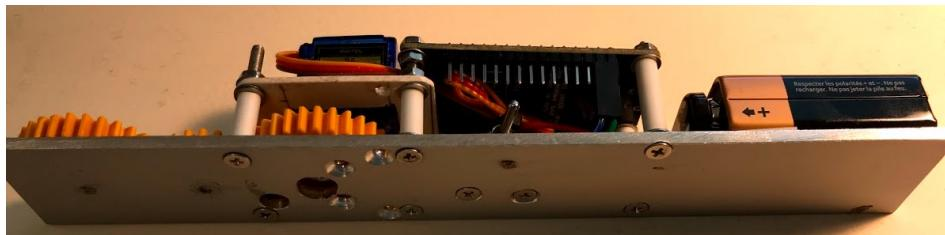
Metal plate – 31 x 200 x 3 mm. The weight of the plate stabilizes the wagon when driving
