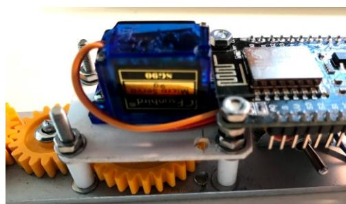
The servo is mounted on a 31 x 44 x 2 mm plastic plate
