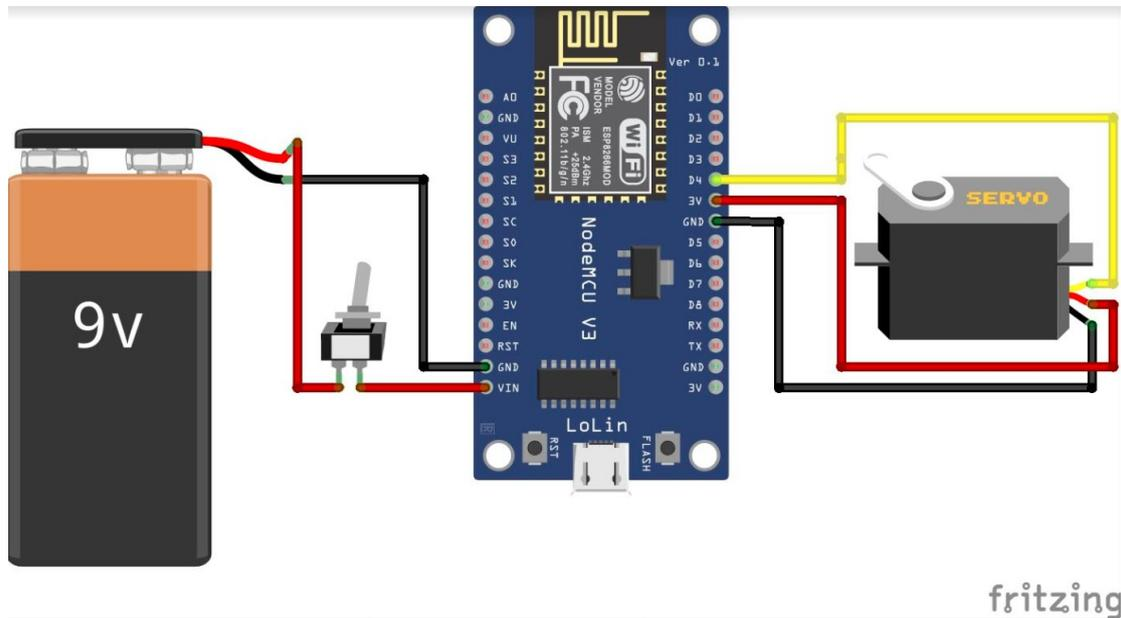
The servo with its three wires is connected in this way:
